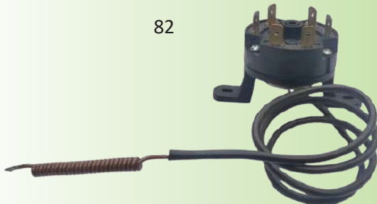
3 pole manual reset high limit thermostat, fail safe, fixed setting, temperature range up to 170°C
